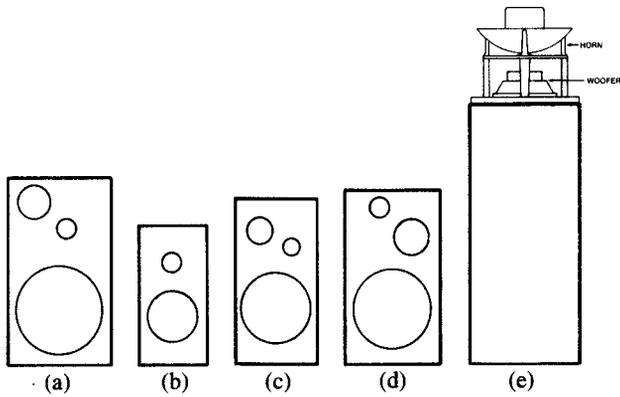
**Fig. 5.** The configurations of the five loudspeakers which were used in the panel test. Speaker (e), the quasi-omnidirectional design, was also used in the localization experiment.
