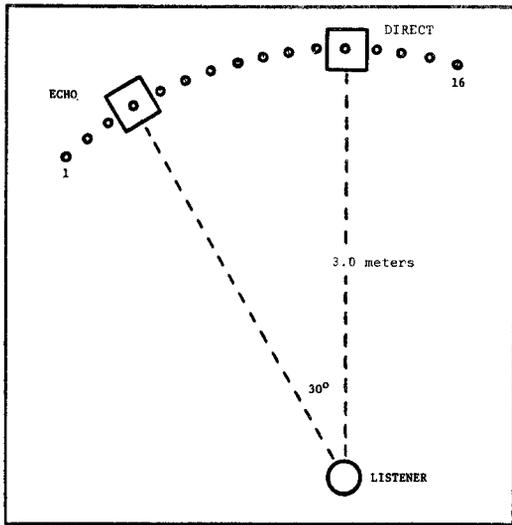
Fig. 1. Two loudspeakers were set up in an anechoic chamber for localization experiments, one representing the direct sound and the other the sound which would be reflected from the wall of a listening room.
