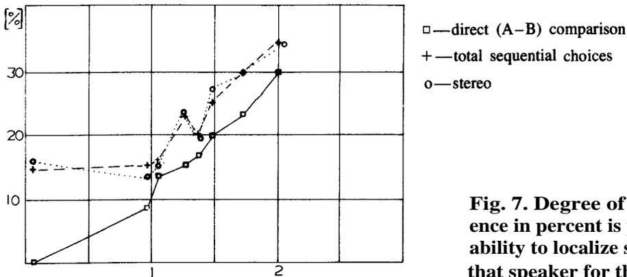
**Fig. 7.** Degree of speaker preference in percent is plotted against ability to localize sound image with that speaker for the panel tests.
