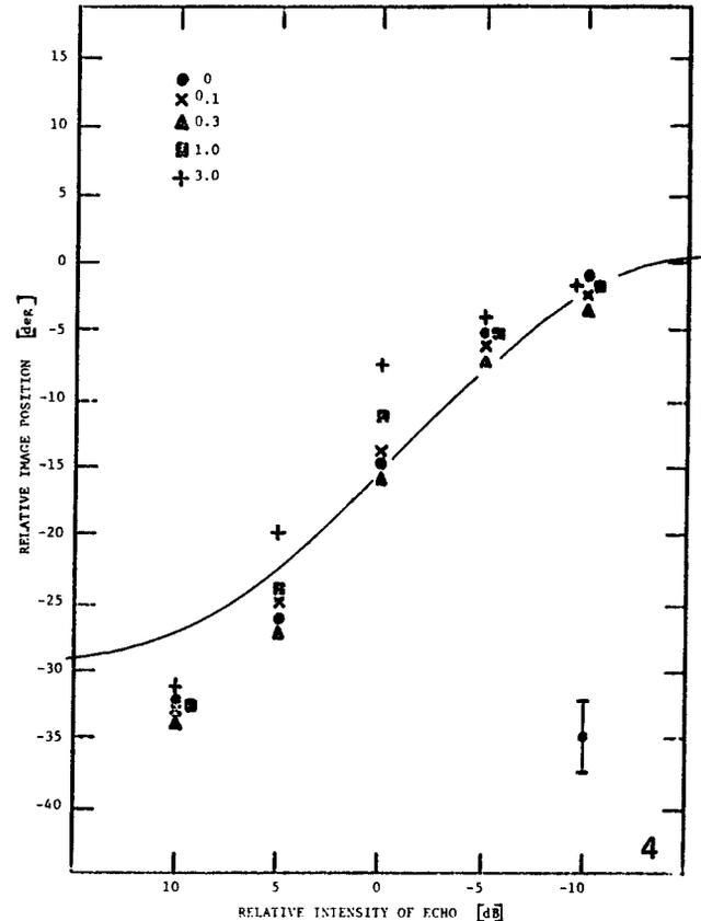
Figs. 2 - 4. Data from the localization experiment is plotted as apparent image position in degrees from the direct speaker versus the relative intensity of the echo speaker for 250 Hz, 1,500 Hz, and 6,000 Hz, respectively. Different shaped points correspond to different delays in milliseconds, as indicated by the legend.
